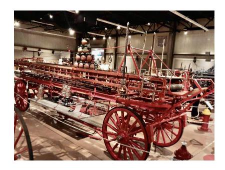
The Hall of Flame's Babcock is notable not only for its rarity and history but also as a masterpiece of restoration. Hall of Flame restorer Don Hale had to re-construct the wheels, axles and the entire front end to bring the piece to its current condition. It makes a majestic sight.
